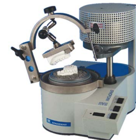
Figure 1. Rapid vacuum thermoforming unit with occludator attached.
